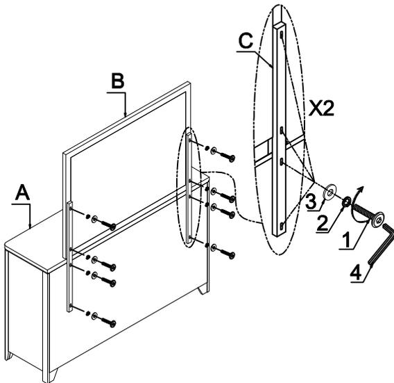
**\*\*DO NOT TIGHTEN BOLTS UNTIL COMPLETELY ASSEMBLED**
