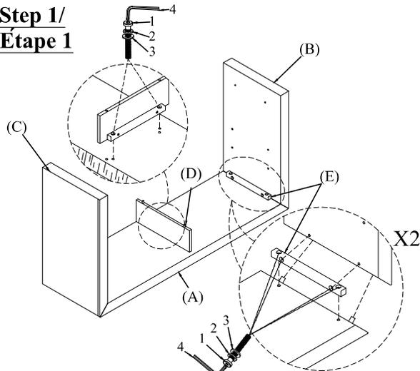
DO NOT TIGHTEN BOLTS UNTIL COMPLETELY ASSEMBLED.
